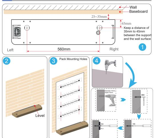
The M6x70 expansion bolts delivered with the battery are mainly used for solid concrete walls and concrete floors. If other types of walls and floors are used, ensure that the walls and floors meet the load-bearing requirements (one battery module weighs 55 kg) and select the bolts by yourself.
